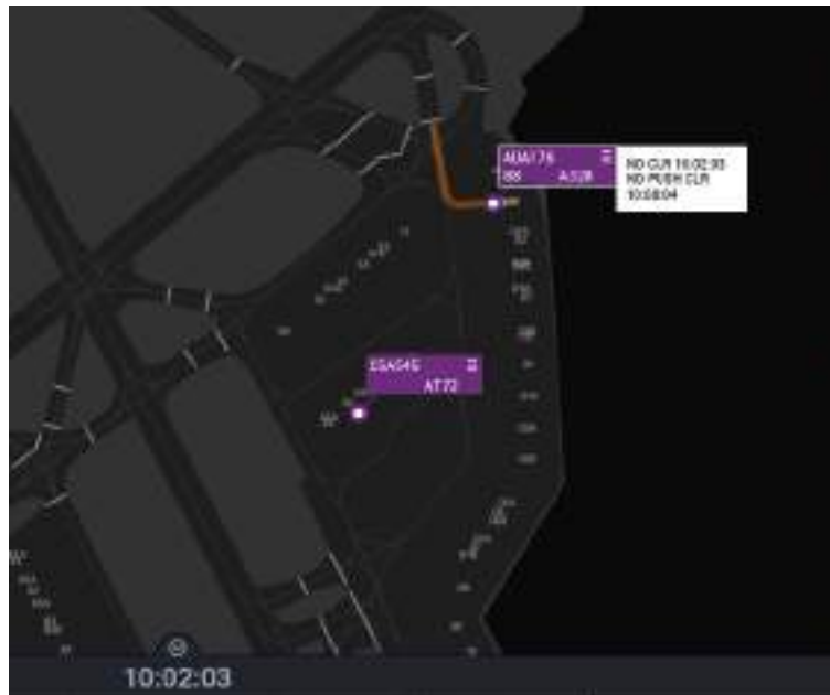
Figure 5.36: Two alerts are raised when AUA176 pushes back without pushback clearance but with taxi clearance
