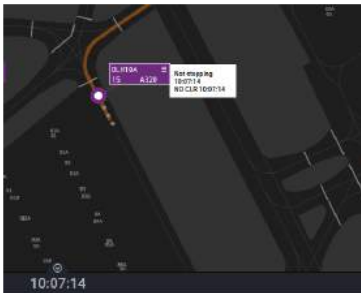
Figure 5.29: An alert is raised when DLH10A does not stop as it should and continues moving with constant speed
