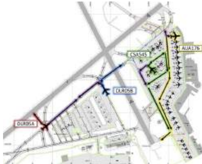
Figure 5.42: Schematic of test situation for route deviations of four AC. The assigned routes are shown in red, blue, green and yellow, the taken ones in purple
