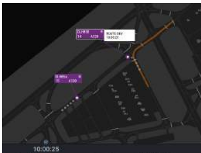
Figure 5.27: Route deviation alert is shown as the AC is taxiing with opposite heading
