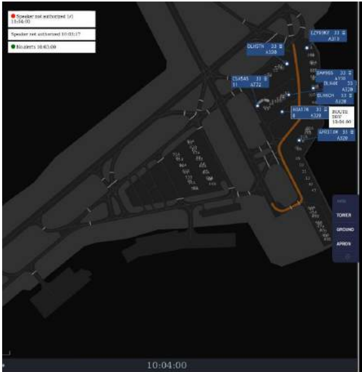
Figure 5.49: Red security situation indicator due to an unauthorized speaker and a route deviation
