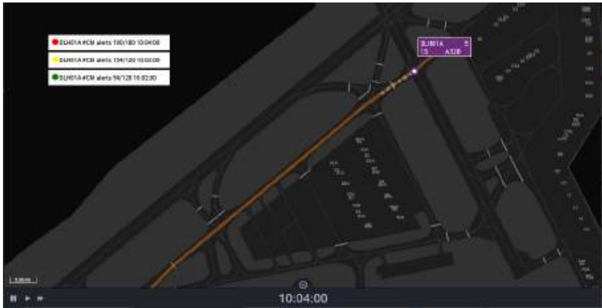
Figure 5.39: An even longer lasting route deviation leads to a red security situation indicator on the ATCO's HMI
