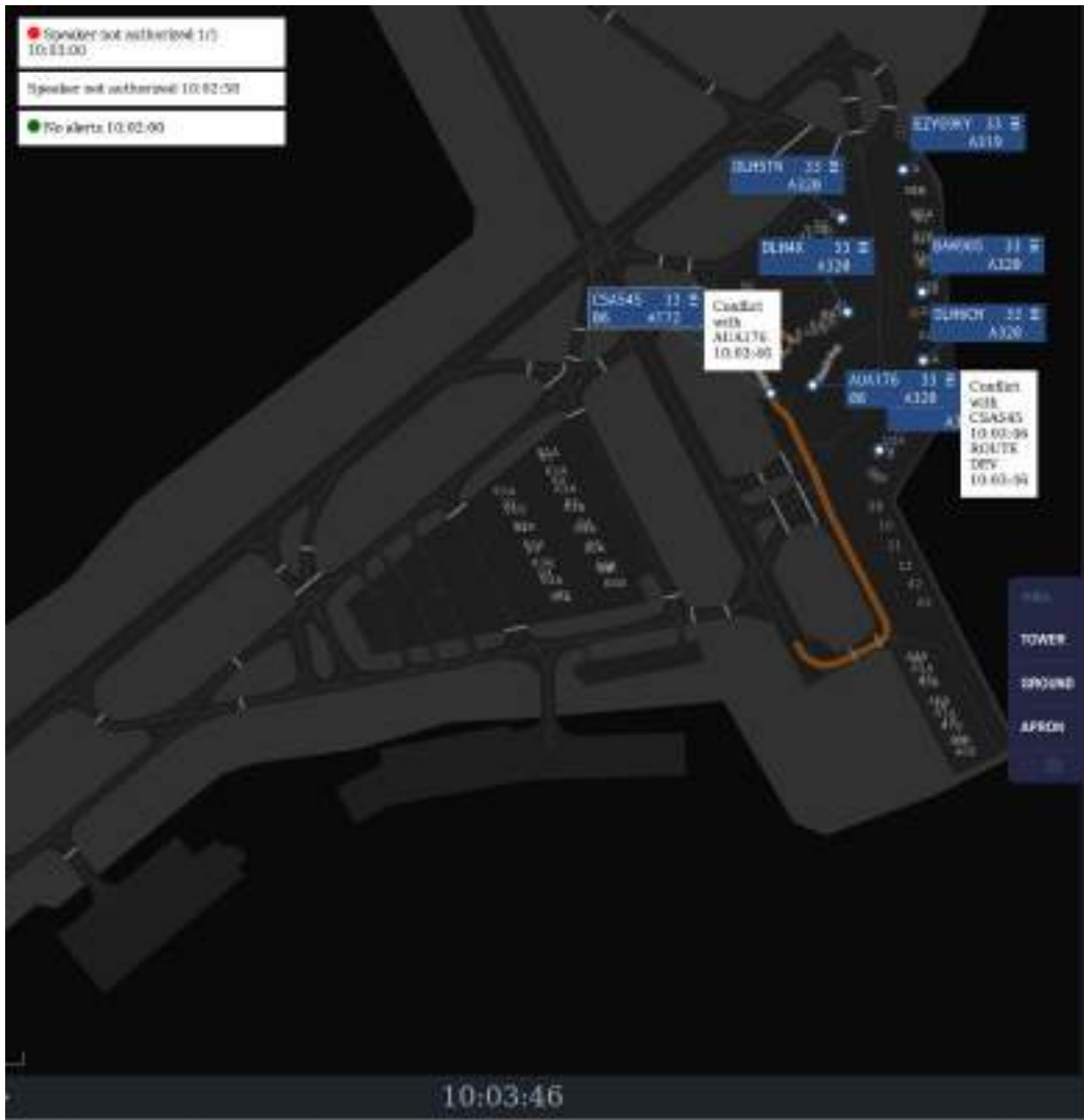
Figure 5.51: A conflict and an unauthorized speaker change the security situation indicator to red
