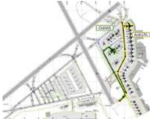
Figure 5.20: Schematic of the test situation leading to two AC taxiing to the runway-holding point
