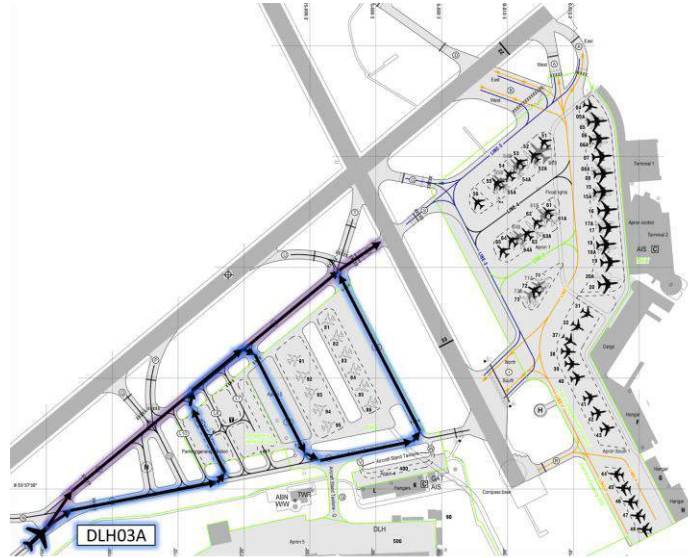
Figure 5.4: Schematic of the test situation to detect multiple route deviations of one aircraft. DLH03A has a planned route, but will taxi differently.
