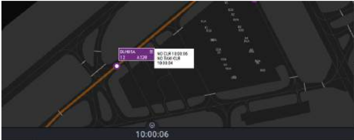
Figure 5.34: Two alerts are raised when an aircraft received line up clearance without taxi clearance
