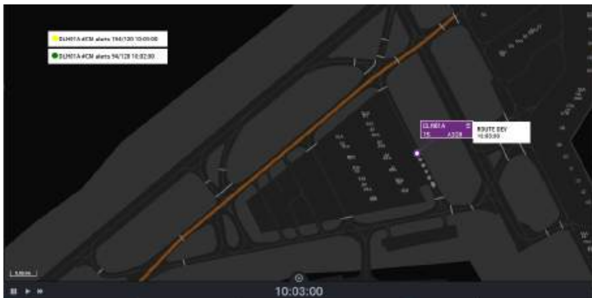
Figure 5.38: A long lasting route deviation leads first to a yellow security situation indicator on the ATCO’s HMI
