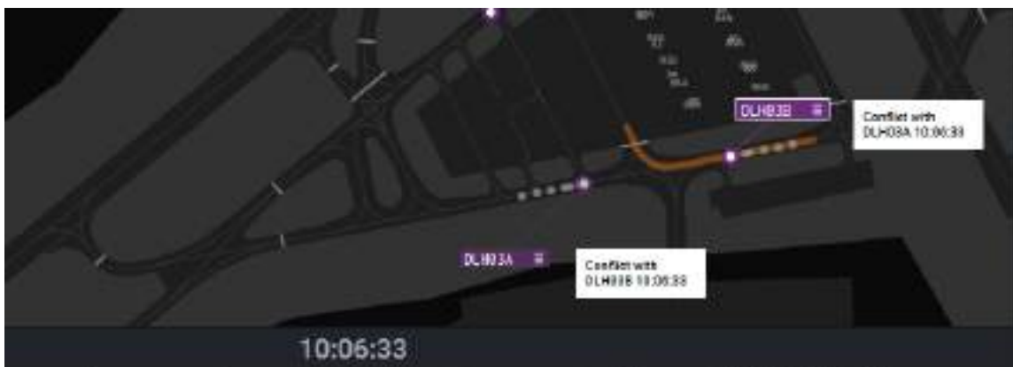
Figure 5.19: Conflict resulting from two AC at a crossing with disjointed routes shown to the ATCO
