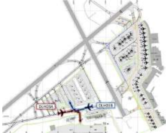
Figure 5.18: Schematic of the test situation for two AC at a crossing with disjointed routes
