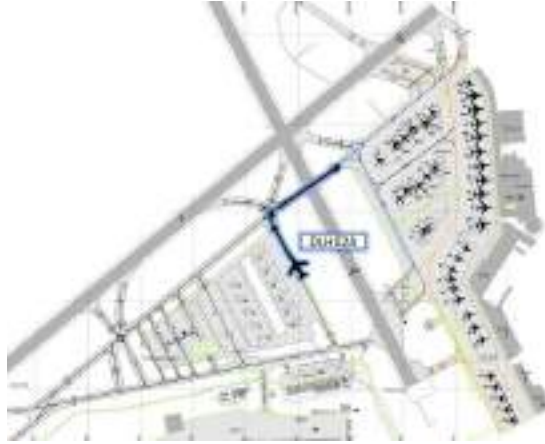
Figure 5.30: Schematic of the test situation for DLH02A which was holding as directed but starts taxi again without continue taxi clearance
