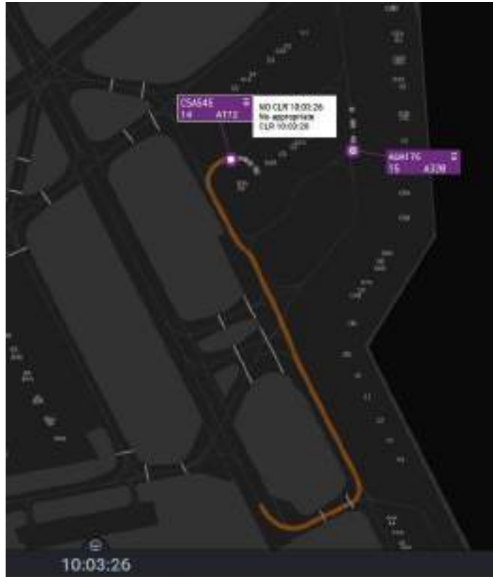
Figure 5.35: Alert for a not appropriate clearance
