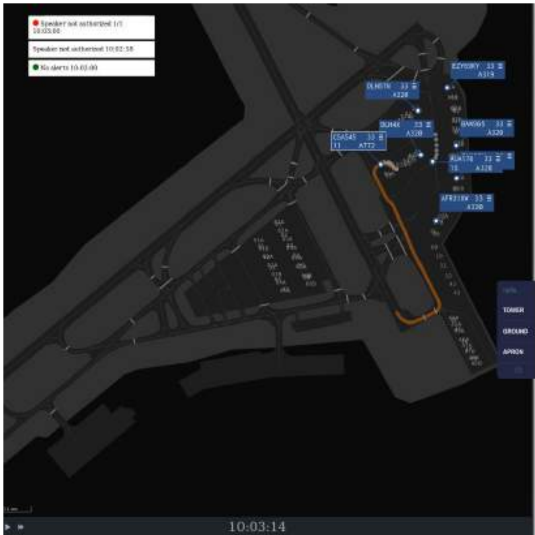
Figure 5.37: The Global Alert List contains the unauthorized speaker alert and the resulting red security situation indicator
