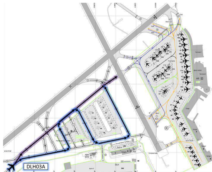
Figure 5.40: Schematic of test situation for multiple route deviations of one AC, which lead to yellow security situation indicator. DLH01A has a planned route, but will taxi differently
