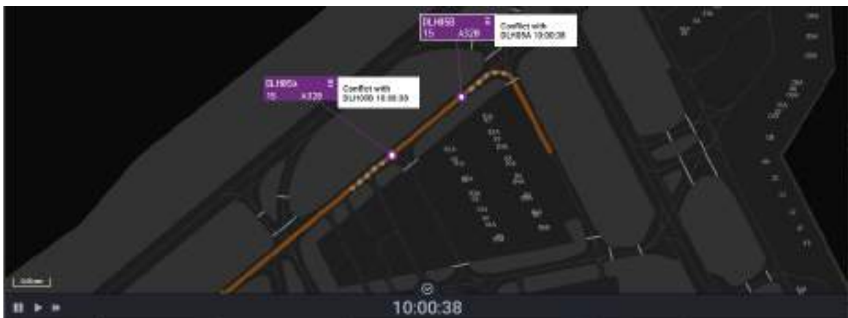
Figure 5.11: The conflict alert resulting from opposite traffic at a crossing is shown to the ATCO
