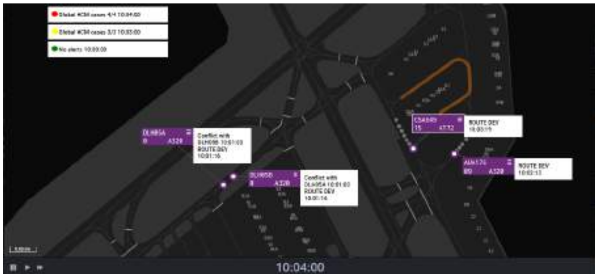
Figure 5.43: Route deviations of four AC lead to a red security situation indicator
