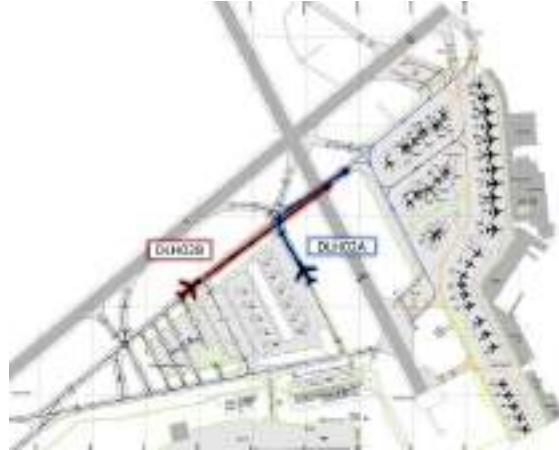
Figure 5.14: Schematic of the test situation for two AC at a crossing merging into the same taxiway. DLH02A stops correctly at the stop bar.
