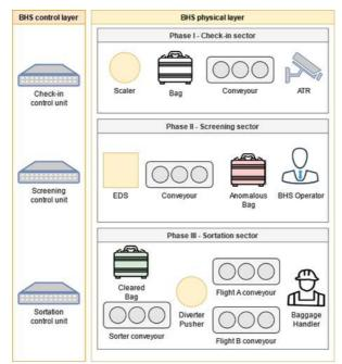
Figure 2.8: Example of BHS Distributed Control system
