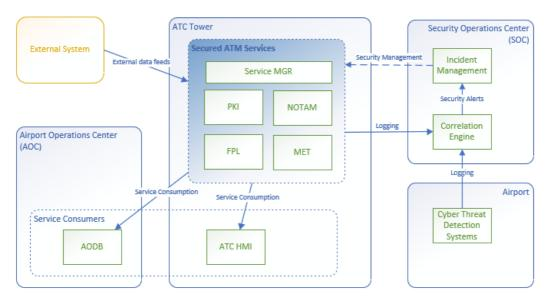
Figure 3.2: Interfaces of Secured ATM Services
