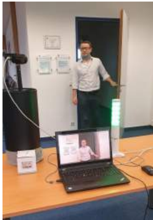
Figure 3.8: Photo of the Unified Access Control system deployed for the demo at AIA with camera, LED tower feedback and Augmented Vision computer
