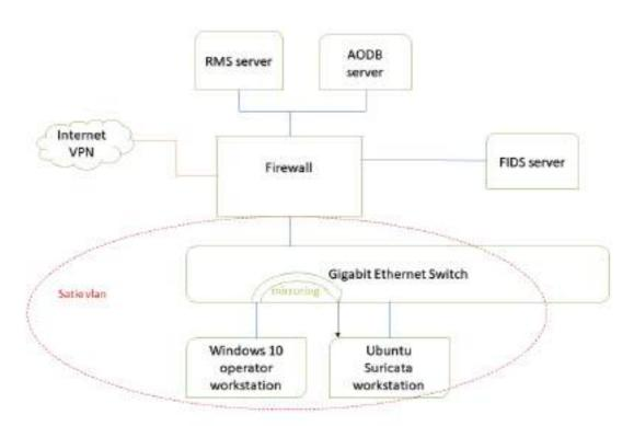
Figure 2.16: Network configuration with mirrored port
